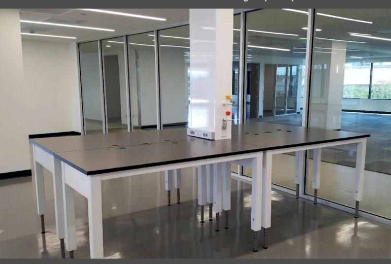
Workbenches and shelves are produced by CNC machines from anti-UV and acid resistant compact laminate plates.
