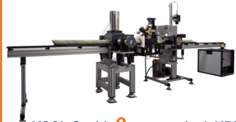
MSCL-S with 9 sensors incl. XRF
